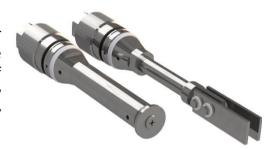
The Axess AXHP range of coupon holders are designed for use with our AXHP access systems and allow the insertion and removal of corrosion coupons in pressurized piping systems up to 10,000psi. The coupon holders are installed through permanently mounted access fittings allowing installation and replacement of coupons without the requirement to isolate process pressure avoiding expensive isolation and shutdowns.
