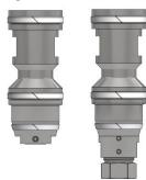
The Hollow or Solid Plug provides the pressure seal in the access fitting and is the carrier for the corrosion monitoring device (probe or coupon holder). The primary packing and guide rings are made from PTFE (15% glass filled) as standard but are available in a range of materials including metal seals for high temperature service.
