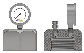
Lighter duty covers in vinyl or carbon steel are available for thread protection during transport and installation only. Axess recommends all HP Access Fittings, once commissioned, are installed with Pressure Retaining Covers.
